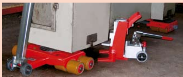
Castors with ball bearings guarantee easy movement
